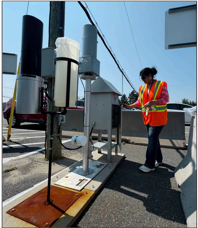
SNOLAB Scientific support staff Dimpal Chauhan changes out the filter at Health Canada's Canadian Radiological Monitoring Network at SNOLAB.
