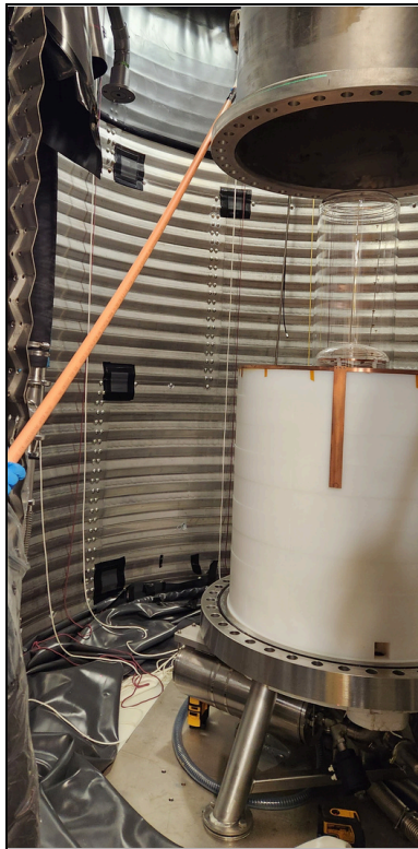
ABOVE: The most recent fill of the PICO-40L chamber with 70 kg of refrigerant, after which a single bubble event was captured during the commissioning of the pressure system.
