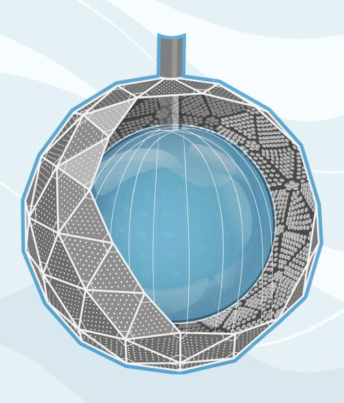
SNO+ uses a liquid scintillator to detect neutrinos. When a neutrino hits the detector, it creates charged particles that cause the scintillator to give off light which is detected by thousands of sensors surrounding the vessel.
