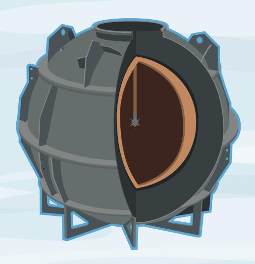
NEWS-G uses a spherical copper vessel filled with a noble gas to search for dark matter. When a particle enters the sphere it ionizes some of the gas, creating electrons.
