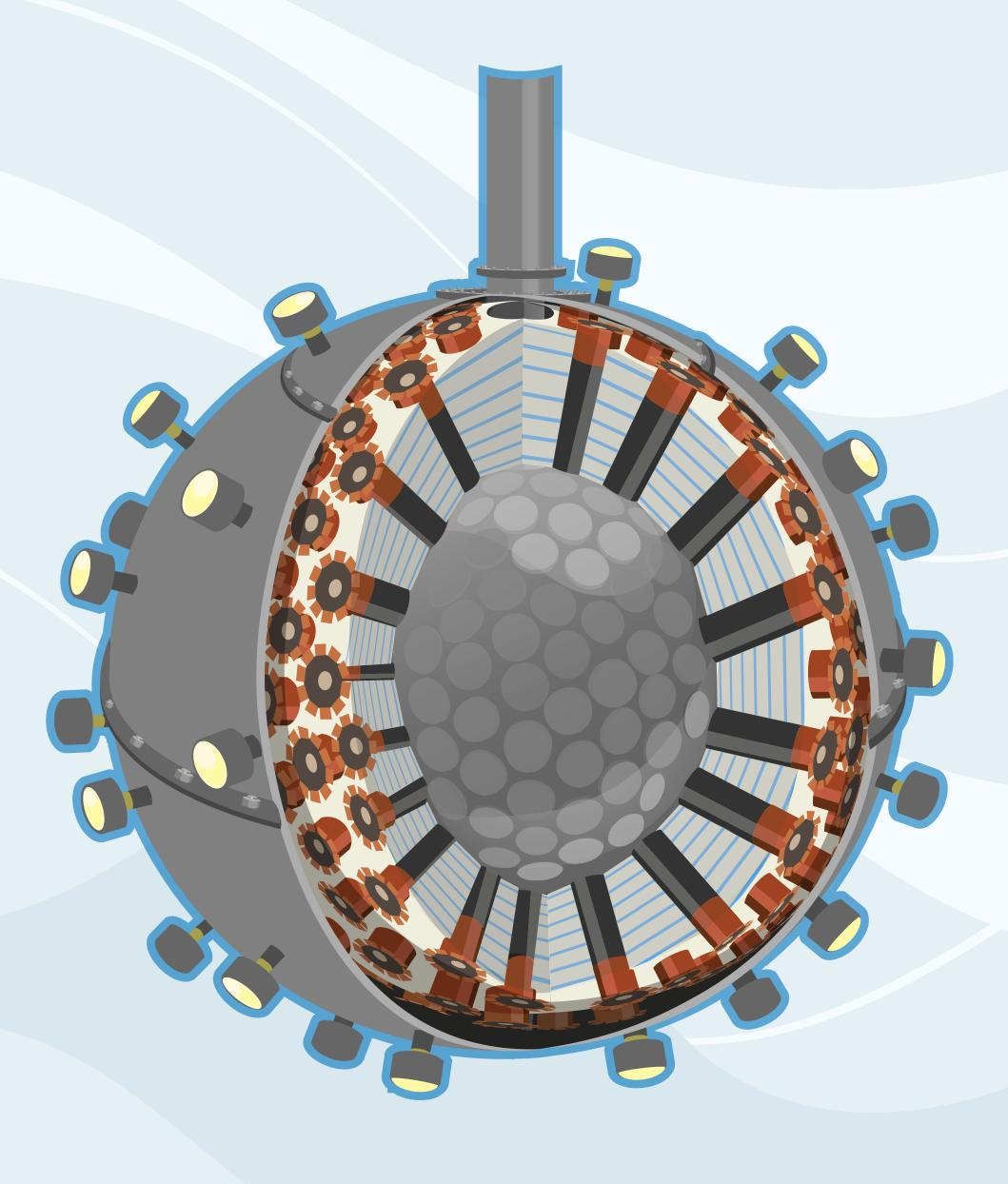
DEAP-3600 uses a vessel of liquid argon to look for dark matter by sensing the ultraviolet light produced when the argon atoms are excited by particle interactions.
