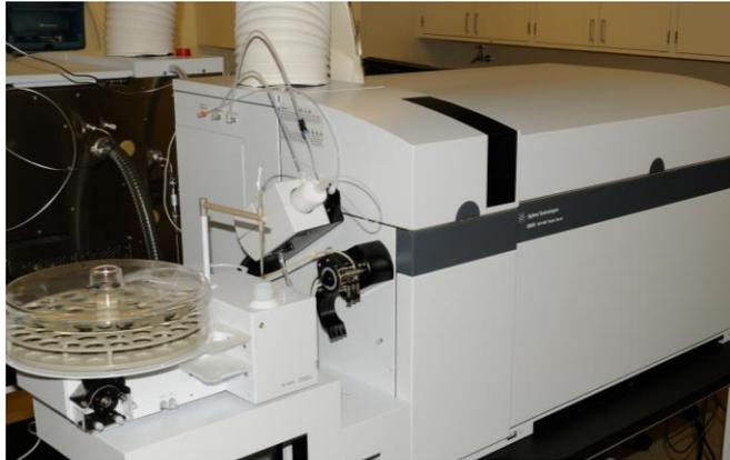
Two dedicated ICP-MS instruments for physics assay for ultra low  $^{40}\text{K}$ ,  $^{232}\text{Th}$ ,  $^{238}\text{U}$ , etc. CASCADES 14-Crystal HPGe Spectrometer, variety of others
