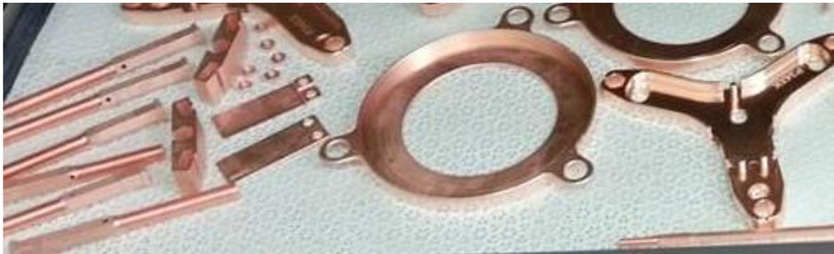
Cu parts for  $\beta\beta(0\nu)$  experiment, The Majorana Demonstrator, are purified and produced through Electroforming at both PNNL and SURF
