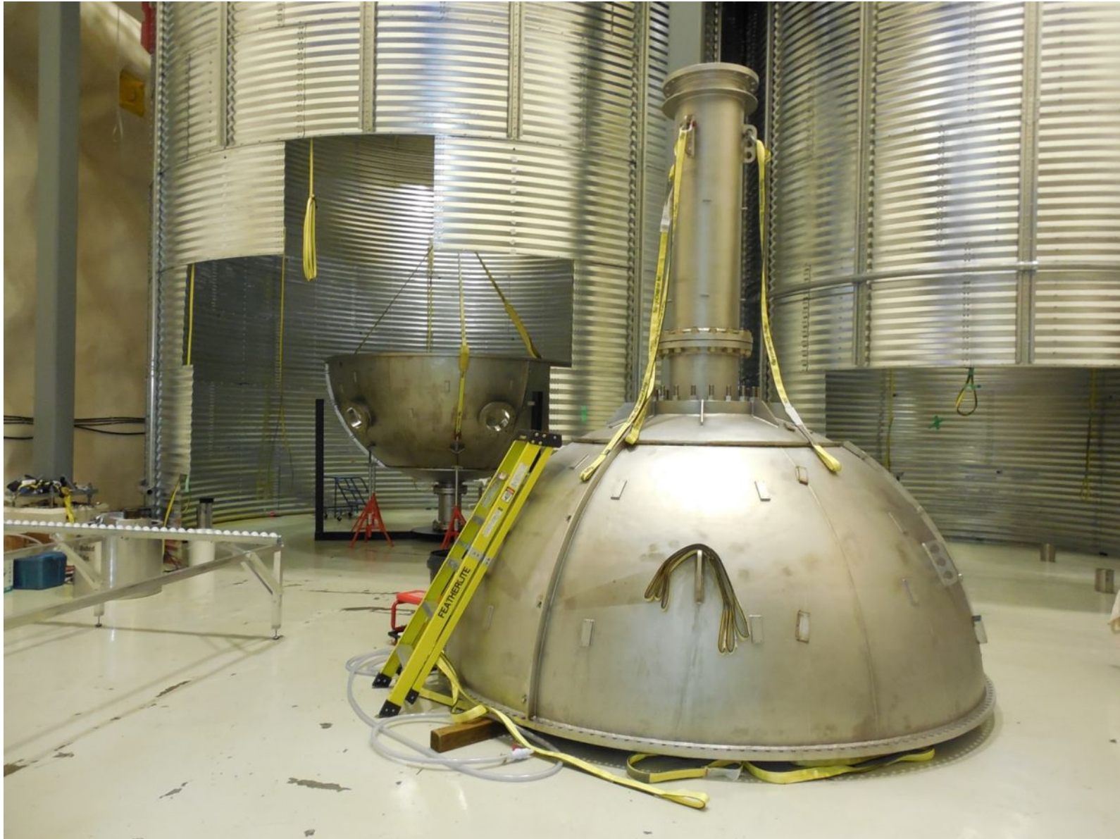
Top and Bottom Steel Shell Hemispheres in SNOLAB Cube Hall (Dec. 2012)
