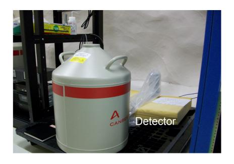
2. SOUDAN Gopher HPGE detector, shielding base is assembled, awaiting lead and copper shielding, the low background lead is has just been cleaned.
