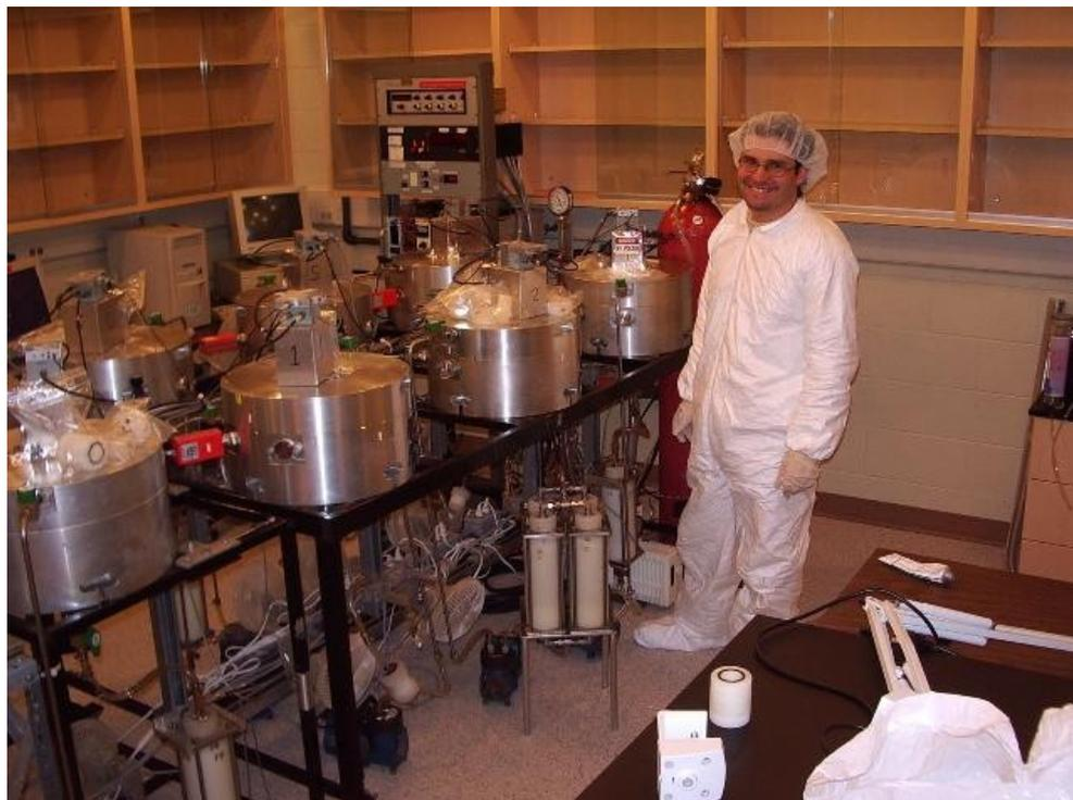
Originally built for SNO, now used primarily by EXO. However, these counters are owned by SNOLAB so samples can be measured for other experiments.
