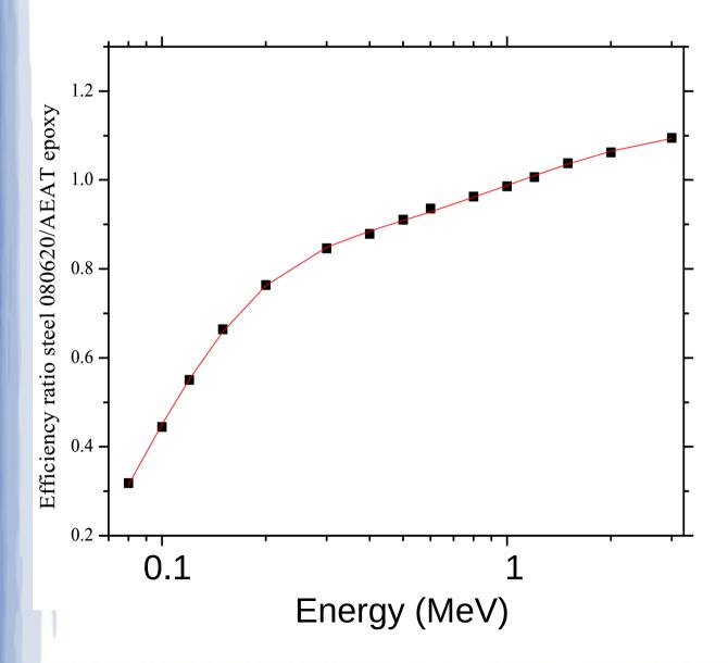
Efficiency correction for steel sample.
