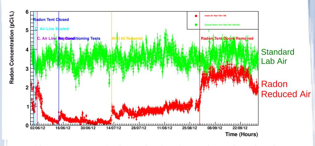
With proper controls the radon levels can be reduced to that of the input compressed air.
