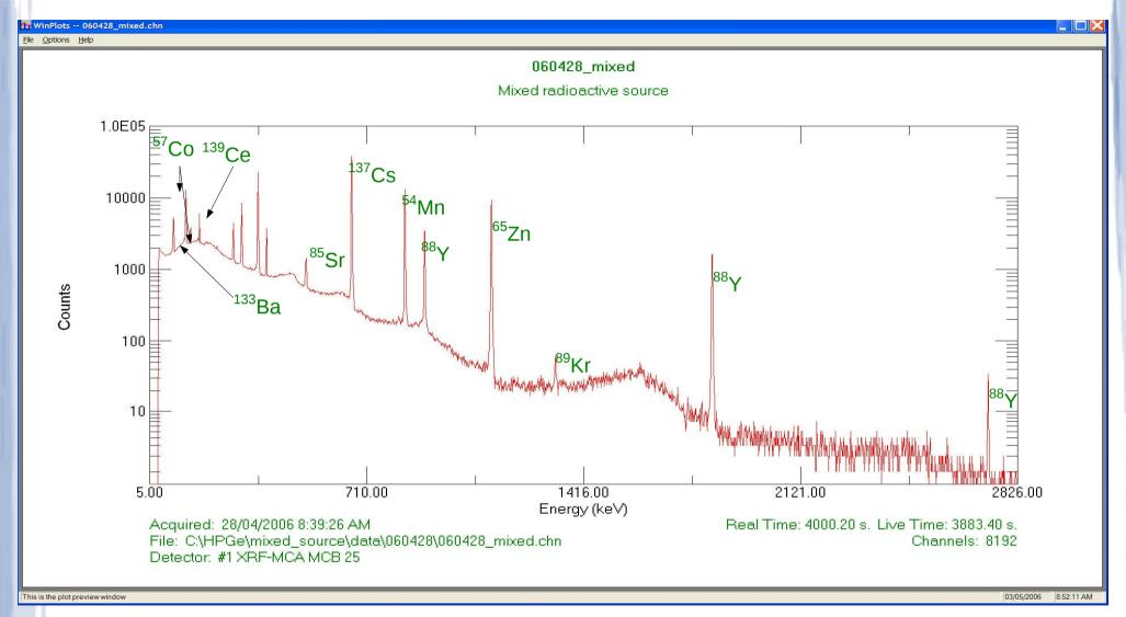
New calibration standards are being proposed which have much longer half-lives to allow the calibration sample to be used for several years unlike most commercial multigamma calibration samples. Would be used to cross-calibrate PGT and Canberra detectors.
