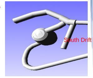
Increased air flow and perhaps other radon reduction techniques will be used. It is known that the compressed air from surface has substantially less radon than the lab air and can be used to reduce radon levels from 135-150 Bq/m³ to 1-5 Bq/m³.
