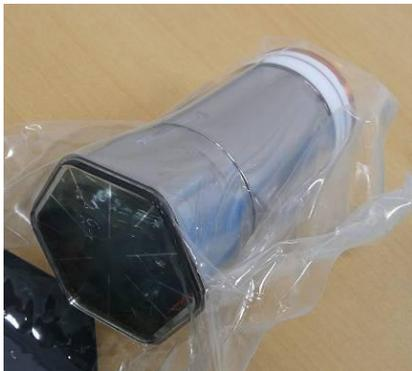
We developed new ultra low RI PMT with Hamamatsu. (1/100 of ordinary one).
