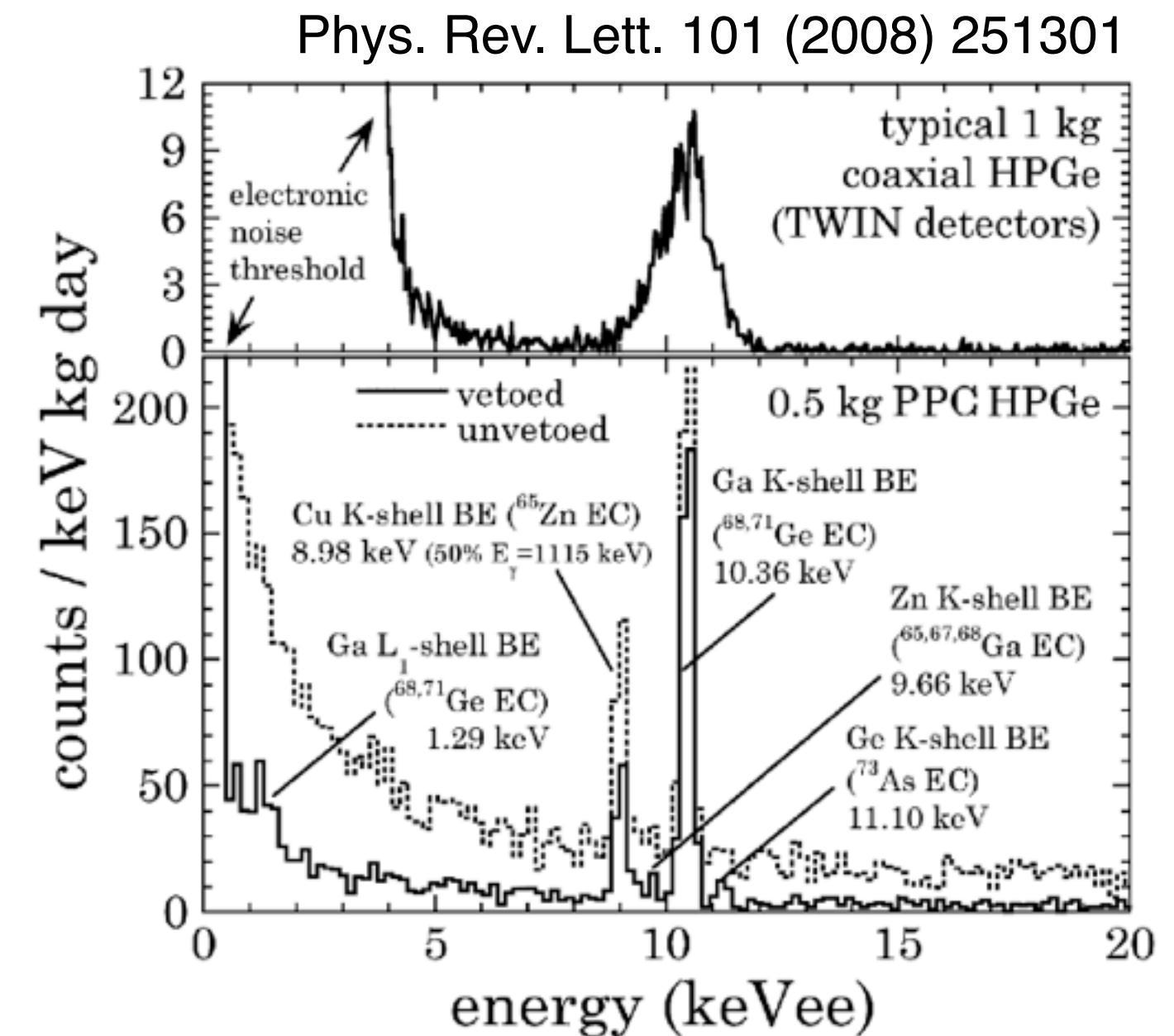
Intrinsically low capacitance, low noise, low threshold
