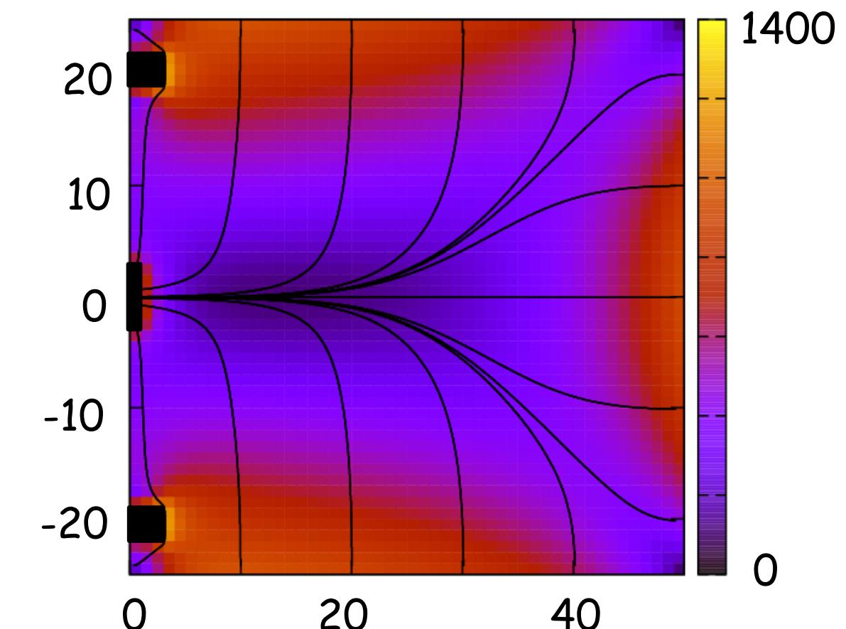
Too wide: loss of characteristic signal shape, poor charge collection
