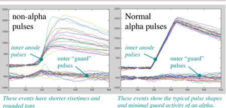
**Above:** The position and type of particle affect the shape of the recorded pulses. Tracks originating from the edges of the counting region and chamber sidewalls show significant outer electrode activity and are rejected. Tracks originating from the ceiling or volume of the chamber exhibit short risetimes, low energies and/or rounded tops.
