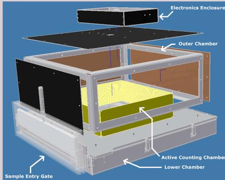
**Above:** The detector is a large ionization chamber. The inner (counting) chamber is filled with Ar gas. Samples are placed on a large 20"X20" tray at the bottom of the chamber. Ionizing particles produce tracks, which are collected on inner and outer (concentric) electrodes.
