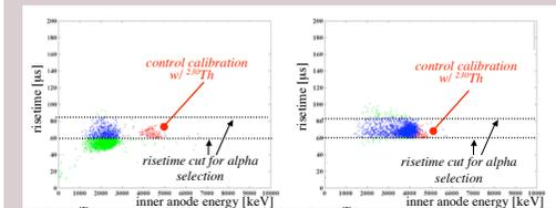
**Above:** These plots show the effect of counting a material with a high moisture content. In the left plot, a sample of 1/4" teflon lines the sample tray during a <sup>230</sup>Th calibration. The blue events show that the energy and the risetime are degraded compared to a control calibration run (no teflon). In the right plot, the same 1/4" teflon lines the tray during a <sup>230</sup>Th calibration run, but after drying the teflon in the chamber with the Argon purge for 4 days.
