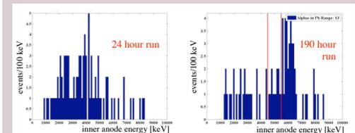
**Above:** Early studies also indicated that the steel tray was a significant source of alphas. Lining the tray with a very thin, 2 mil, layer of teflon significantly reduced the background from the tray. The plot on the left shows a run taken with the empty steel tray. The plot on the right shows a longer run taken with teflon lining the tray. Note the right and left plots are not normalized by exposure time.
